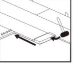
Step 7: Tap end of plank with hammer and tapping block to lock ends of planks together. Remove support bridge and continue with this method until you have completed installing the row.
