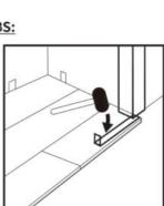
Step 2: Use hammer and pull bar to draw and lock short end of plank.
