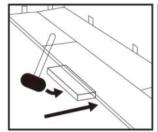
Step 5: IMPORTANT! Use a hammer and tapping block to tap the long edge of the plank to ensure a tight fit. Note: Tapping block should be a minimum of 10" to 12" long. It is important to note that any/all gapping can/will compromise the locking system.
