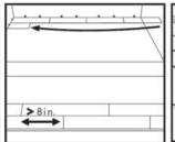
Step 3: Use the remaining plank from your cut piece to begin the next row (you will repeat this process throughout the installation). Note: It is recommended that you space end-joints by a minimum of 8 inches.
